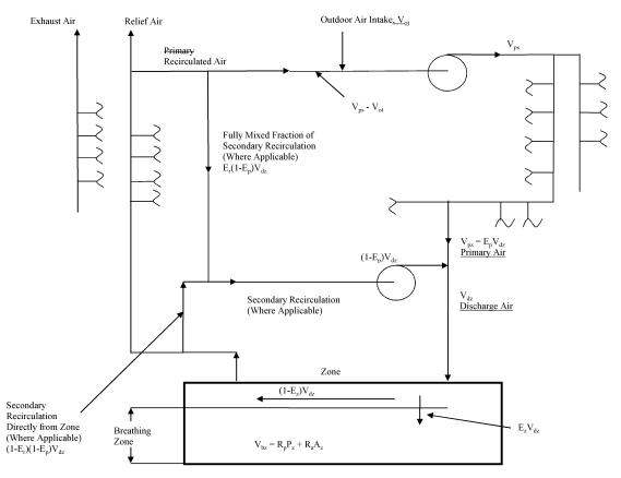
Figure A.1 Ventilation system schematic.
